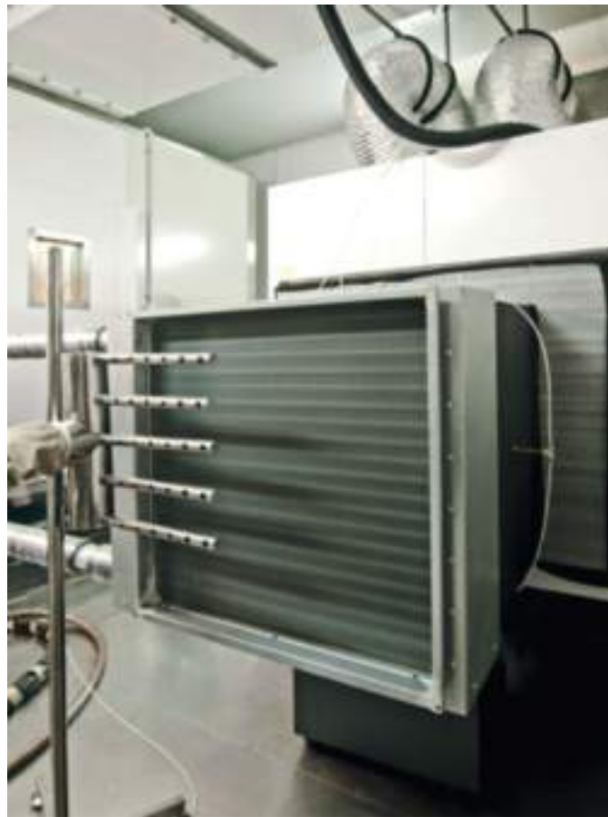
Chart 6: Test setup for heat exchanger tests acc. to ASHRAE standard 33-2000
