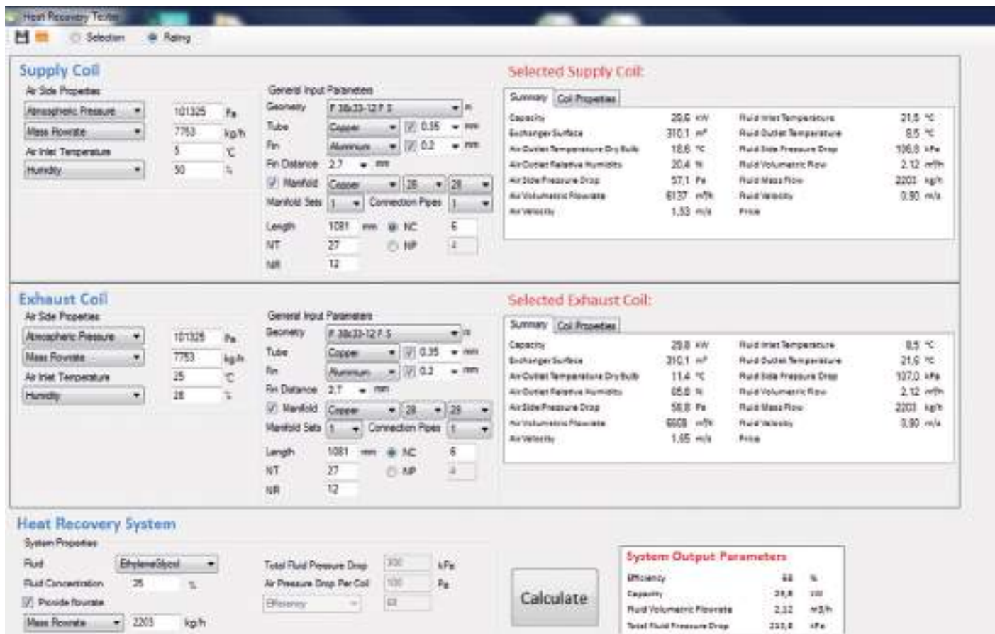
Chart 5: Internal Friterm software for coil energy recovery loop systems
